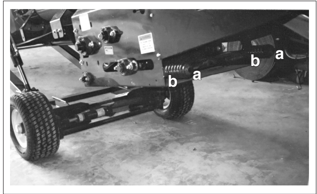
Fig. 48 CONVEYOR BELT TENSIONING SPRING
