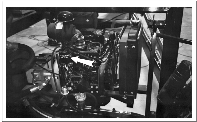
Fig. 64 FUEL FILTER - 85 FOOT MODEL
